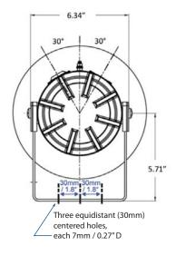
\* All versions are fitted with one (1)  $\frac{1}{2}$  inch NPT entry and two (2) 20mm entries. All entries are fitted with brass stopping plugs as standard.
